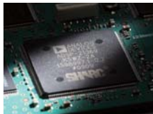
<DSP unit> ADSP-21369 Internal clock speed: 333MHz 32-bit floating point DSP Max. performance: 2000MFLOPS
